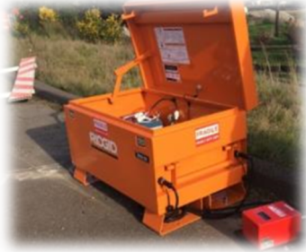
Figure 6: Mounting with rugged enclosure + batteries (options)
