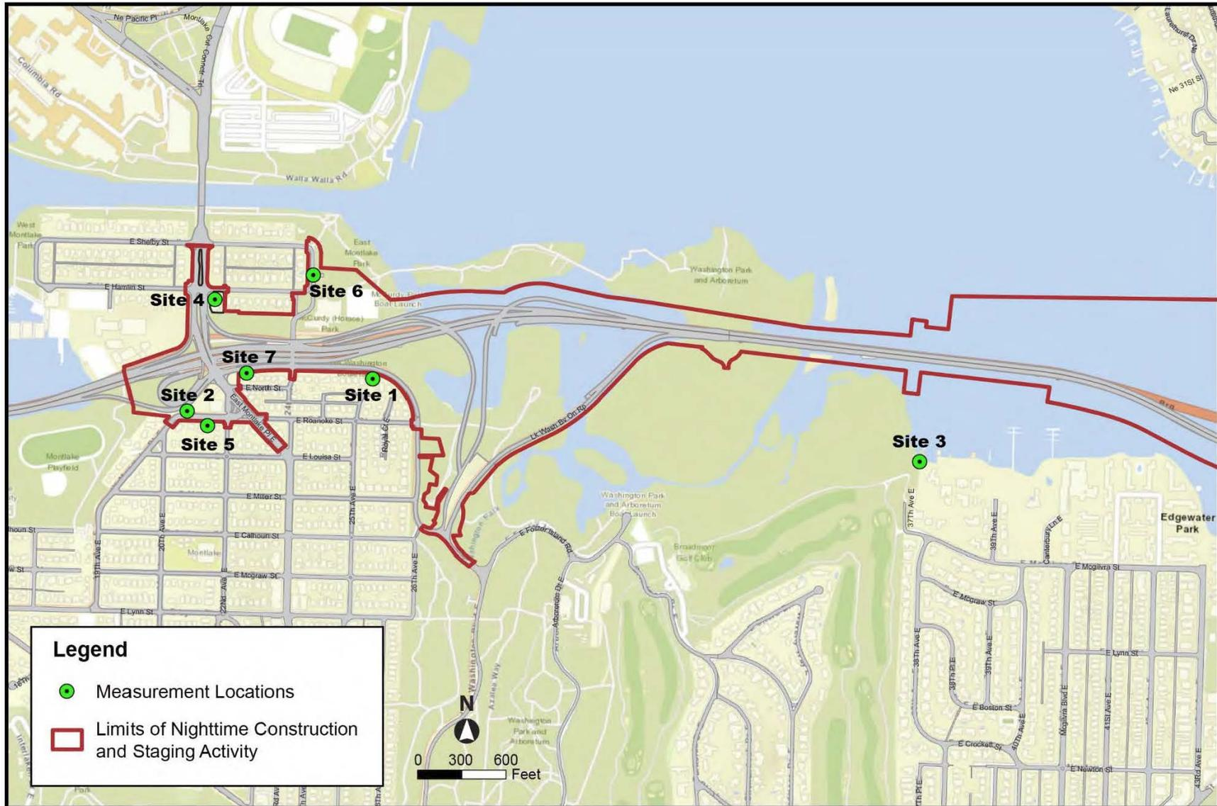
In addition to the  $L_{eq}$ , this noise variance application proposes to track compliance with the terms set by the MPPCNV by monitoring the measured hourly  $L_1$  sound level. The  $L_1$  has been found to be more reliable than the  $L_{max}$ , as stated in the Denny Substation Program Noise Monitoring and Mitigation Plan, revised February 11, 2015:
