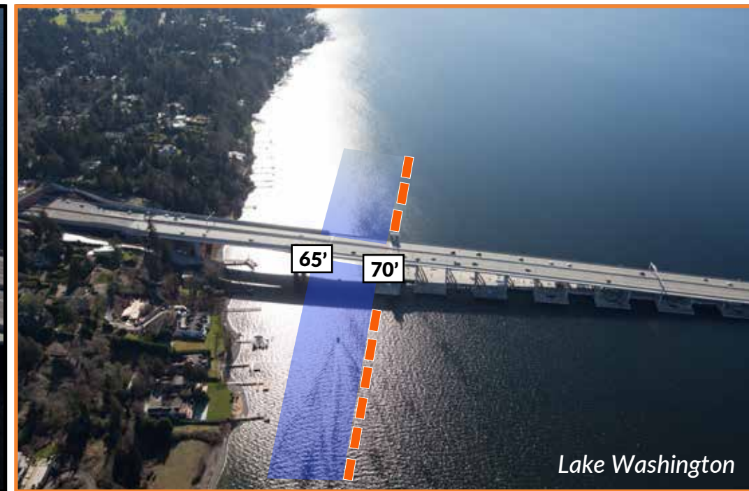
Due to seasonal lake level changes, the east navigation channel height fluctuates between 65 feet and 70 feet
